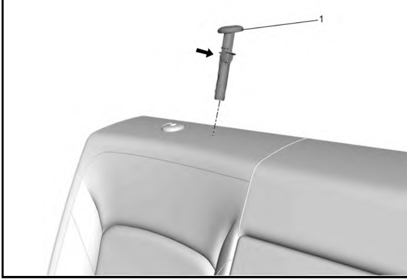
Rear Seat Head Restraint Guide (1) - Install - Rear Seat Head Restraint Guide Replacement
