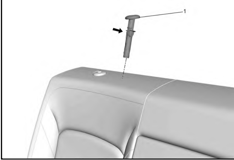
Rear Seat Head Restraint Guide (1) - Remove - Rear Seat Head Restraint Guide Replacement
