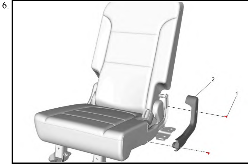
3rd Row Seat Back Hinge Finish Cover (Inboard) (2) - Install - 3rd Row Seat Back Hinge Finish Cover Replacement (Inboard)
