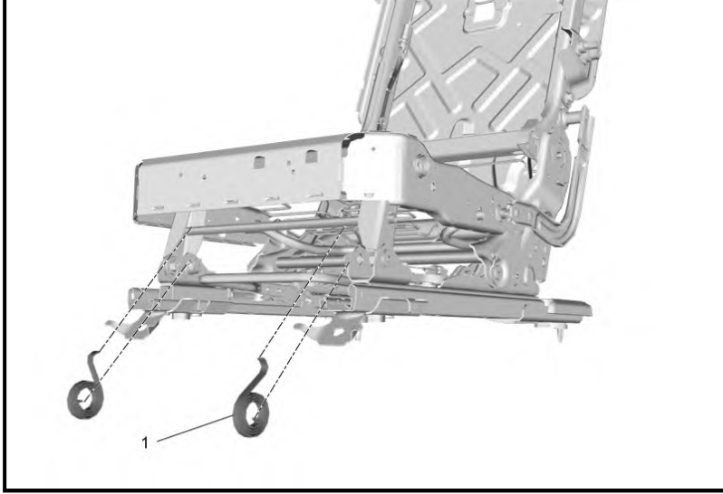
Rear Seat Back Lower Support Wire (1) - Remove [2x]
