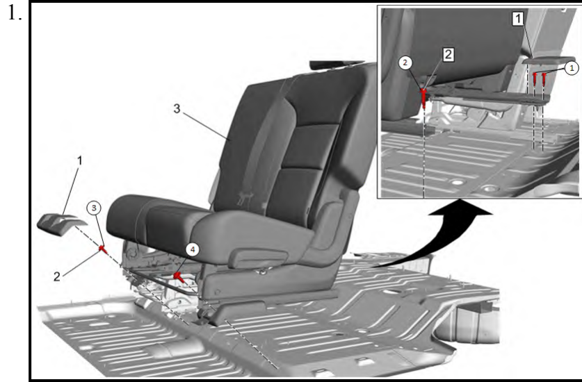
Rear Seat (3) - Remove - Rear Seat Removal and Installation (60%)
