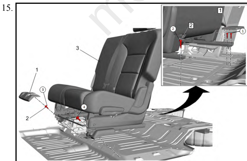
Rear Seat (3) - Install - Rear Seat Removal and Installation (60%)
